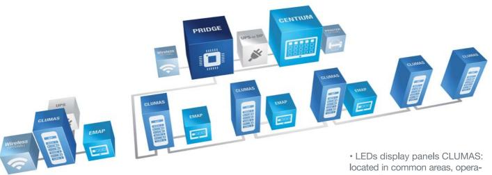
• local control panels EMAPs: placed in ROV and Sat Dive operations offices and Crane operators stations, on which the operating mode is chosen and the DP alarm is validated; in cranes too in order to know when they are operating located in common areas, operations offices, cabins and cranes, which give information about the equipment operation mode
